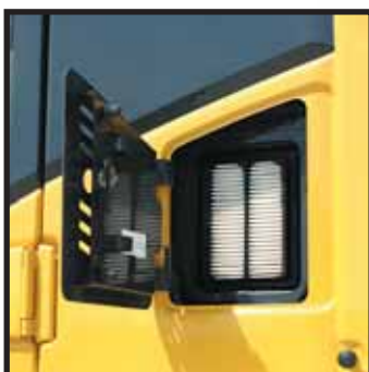
Outer air filter Easy removal/installation of the air conditioner filter element, without tools facilitates cleaning.
